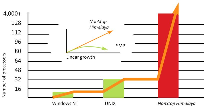
*SMP systems can become impractical, even with as few as eight processors. By contrast, NonStop Himalaya servers can scale linearly to more than 4,000 processors.*
